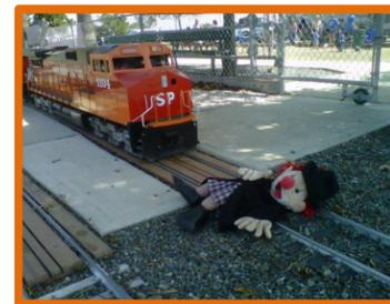
When operating the work engine (public service) to start it you need to be on the left side not sitting on the engine. If sitting on the engine you will probably touch the joy stick causing the engine to jerk forward or backward.
